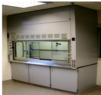
Pictured above is a fume hood. Vanessa Keel of EHS certifies these hoods.
