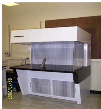
Pictured above is a laminar flow hood. Notice, there is no sash in the front.
